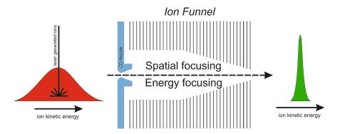
In LAMS, the initial ion-energy distribution from the laser ablation process is very broad; energy focusing with an ion funnel should reduce this distribution to improve transport efficiency through the mass analyzer.
