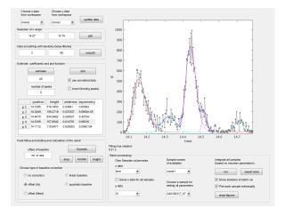
Graphical user interface. Theaxes shows chromatographic data of coffee ( $\Delta t_R = 40$  s). The signals are very noisy and overlapping. Five compounds were automatically detected and fitted in approx. 0.5 s.
