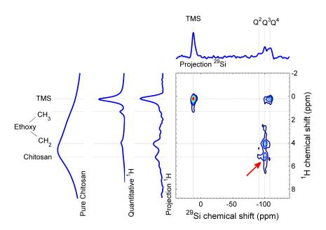
Figure 1. Solid-state <sup>1</sup>H-<sup>29</sup>Si heteronuclear correlation NMR spectrum of a chitosan-silica aerogel hybrid. The red arrow points to the strong correlation between the chitosan protons and the silica surface (Q³); the other cross peaks are typical for silylated silica aerogels.
