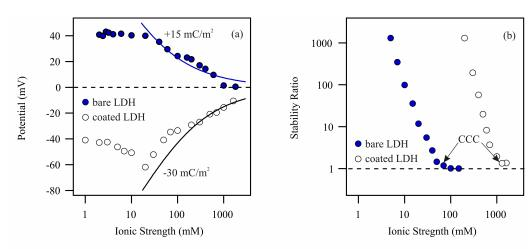
Fig. 1. Electrokinetic potential (a) and stability ratio (b) values for the bare (filled symbols) and heparin coated (empty symbols, at a dose of 100 mg/g) LDH particles at different ionic strengths. The solid lines in (a) indicate the potentials calculated using the Debye–Hückel model.
