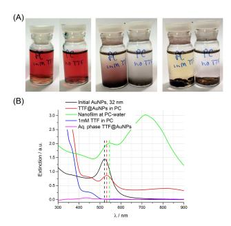
**Figure 1. (A)** Photographs of PC-water system. From left to right: before, right after shaking, and after complete phase separation with and without TTF in the PC phase at the bottom. **(B)** UV-Vis spectra of the initial solutions, the spectra of the aqueous and PC phases after complete phase separation and the extinction spectra of nanofilms formed at the given LLI.
