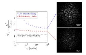
Dynamic rheological measurements and confocal images of fluorescent silica particles partially dispersed in PDMS by Ultra-Turrax mixing at different intensity.
