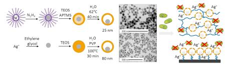
Fig. 1: Synthesis and antimicrobial  $Ag^+$  release of  $Ag@SiO_2$  nanorattles: microemulsion method (top) and Stöber conditions followed by surface protected etching (bottom).
