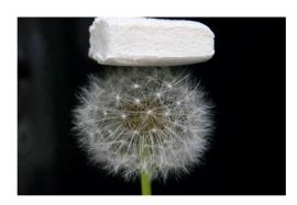
Fig.1 : Ultra light 3D nanofiber based aerogels
