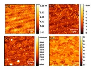
Topography of glass surface functionalised with PAMAM monolayer (a) covered with Jaggregates in plate-like (b) and in monolayer form (c) Phase image showing the Jaggregates in monolayer (d).
