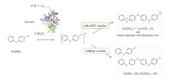
Scheme 1: Illustration of the laccase-catalyzed oxidation and oligomerization of PADPA at pH = 3.5. At the top, the main product of the reaction the presence of AOT vesicles is shown: The green PADPA dimer in its half-oxidized, half-reduced state with spectroscopic similarities to PANI-ES. At the bottom, two hydrolysis products formed in the absence of vesicles are shown (not obtained with vesicles).
