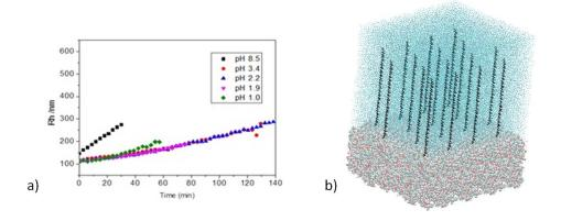
**Figure 1.** Hydrodynamic radius of dispersed particles as a function of time for different pH value, after addition of 0.2 % of SDS (a); molecular model of PMMA surface (transparent VdW spheres) grafted with PAA chains (black residues) in explicit water (blue dots) (b). Explicit ions are here omitted for the sake of clarity.
