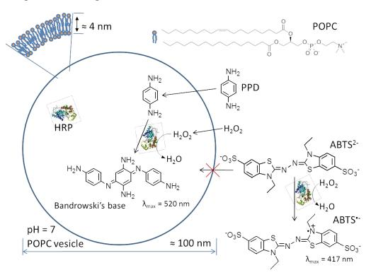
Figure 1: Illustration of the assay system for the spectrophotometric determination of the activity of phospholipid vesicle-entrapped HRP with PPD as substrate and  $H_2O_2$  as oxidant. ABTS<sup>2-</sup> can not permeate the phospholipid bilayer and is only oxidized by non-entrapped HRP. POPC: 1-palmitoyl-2-oleoyl-sn-glycero-3-phosphocholine.
