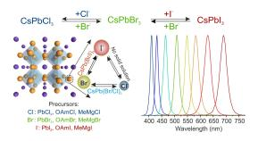
Figure 1: Anion-exchange in the colloidal semiconductor  $CsPbX_3$  perovskite nanocrystals and the tunability of the bright emission over the entire visible spectral region via anion-exchange.
