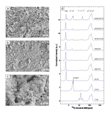
Figure 1. SEM of silica aerogel topography after modification with a) monofunctional b)difunctional c) trifunctional alkoxysilane d)<sup>1</sup>H-<sup>29</sup>Si cross polarization NMR spectra of silica aerogels hydrophobized with various hydrophobization agents.
