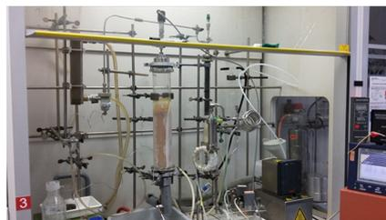
Figure 2. Catalytic reactor and set-up.
