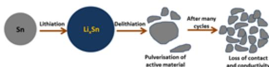
Figure 1: Pulverization of the active material
