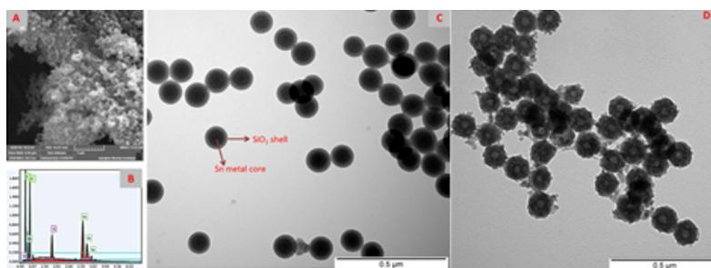
Figure 3: SEM (A), EDS (B) and TEM (3C) showing core-shell Sn@SiO<sub>2</sub>, 3(D) showing Sn@SiO<sub>2</sub>@C after thermal treatment
