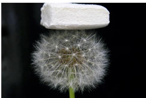
Fig.1 : Ultra light 3D nanofiber based aerogels
