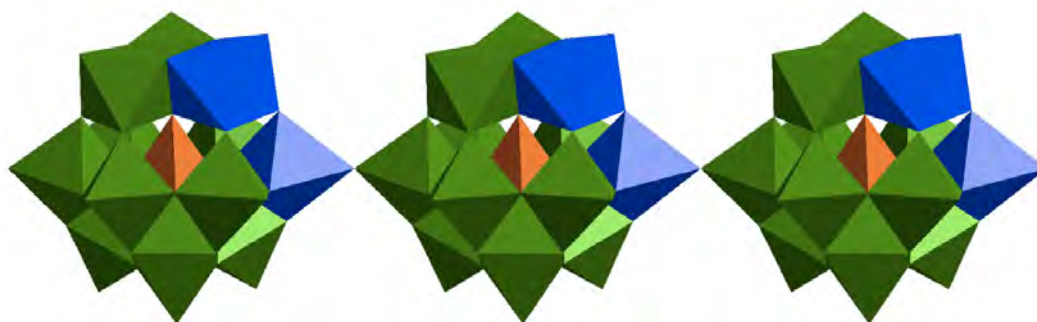
Polyhedral representation of the 1D chain of \{Mn_2SiW_{10}O_{38}\} building blocks
