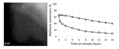
Figure 1: (a) STEM image of the catalyst based on dealuminated zeolite and (b) catalytic activity of the catalysts based on the conventional zeolite (o) and the dealuminated zeolite (r) at  $450^{\circ}$ C in the presence of 5 vol. % water
