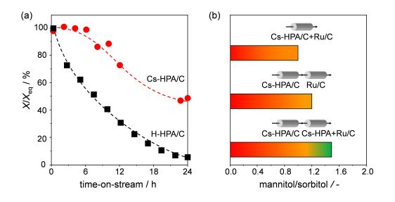
**Figure 1** (a) Extent of epimerization over Cs- and H-HPA/C *vs*. time-on-stream and (b) mannitol/sorbitol ratio upon glucose conversion in different reactor configurations: (i) mixed bed, (ii) sequential Cs-HPA/C and Ru/C beds, and (iii) sequential Cs-HPA/C and mixed beds.
