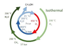
**Figure 1.** Prior high temperature route and the presented isothermal stepped methane to methanol reaction.
