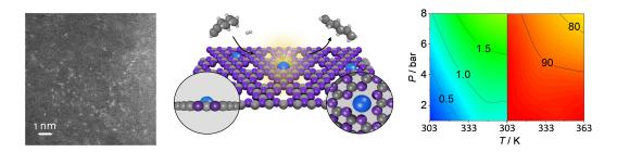
**Figure 1** Aberration-corrected transmission electron micrographs confirm the presence of single Pd atoms in mpg- $C_3N_4$ , which are thought to be stabilized within the 6-fold cavities of the carrier (as illustrated schematically), and exhibit a high reaction rate (in  $10^3 \text{ mol}_{product} \text{ mol}_{Pd}^{-1} h^{-1}$ ) and product selectivity (in %) in the hydrogenation of 1-hexyne to 1-hexene.
