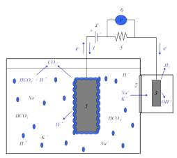
**Figure 1.** MEC for sustainable base generation and important parameters to establish a predictive model. (1) Anode covered by a biofilm composed of *Shewanella oneidensis* MR-1, (2) Nafion<sup>®</sup> membrane N-117 separating the two half cells, (3) platinum sputtered RVC cathode used for hydrogen generation, (4) external power supply, (5) 11 $\Omega$  resistance, (6) multimeter.
