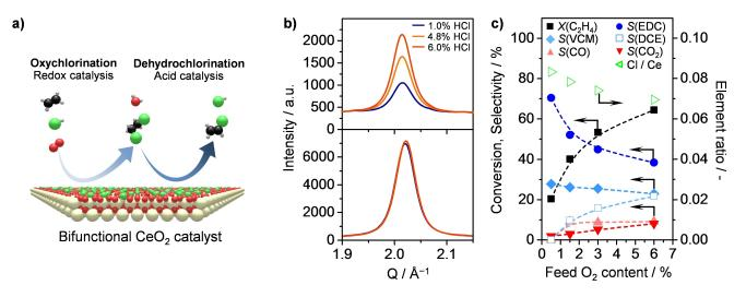
**Figure 1** a) Bifunctional ceria integrates both oxychlorination and dehydrochlorination functions on a single surface for direct VCM production. b) Excerpt of *in situ* SXRD patterns of CeO<sub>2</sub> surface near layers (top) and bulk (bottom). c) Conversion, selectivity, and Cl/Ce ratio *versus* oxygen content in an *operando* PGAA experiment on CeO<sub>2</sub>.
