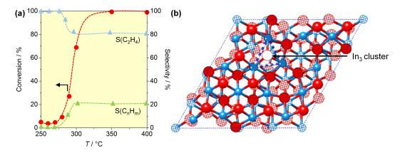
**Figure 1** (a) Conversion (red) and selectivity to ethylene (blue) and to oligomers (green) in the gas-phase semi-hydrogenation of acetylene over  $In_2O_3$ . (b) Illustration of the  $In_2O_3$  structure after surface reduction. Color code: oxygen (red), indium (blue).
