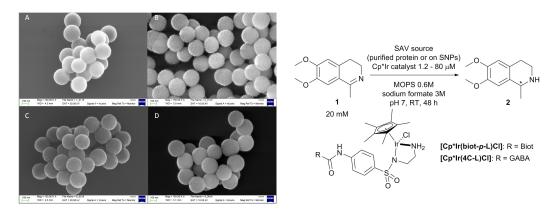
Upon immobilization and protection of streptavidin mutants on the SNPs, the resulting nanoparticles display remarkable catalytic activity with TON = 46000 under the applied conditions for the reduction of 6,7-dimethoxy-1-methyl-3,4-dihydroisoquinoline, with the possibility to recycle the active catalyst. The concentration of the active Cp\*Ir catalyst was determined by means of ICP-MS measurements. This protected system is also able to retain its activity in the presence of cellular debris.
