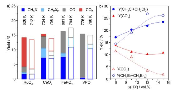
**Figure 1** a) Catalytic performance of oxide and phosphate materials in methane oxychlorination (filled bars) and oxybromination (empty bars) in the presence of 6 vol.% HX. b) Methane oxychlorination (filled symbols) and oxybromination (empty symbols) on  $CeO_2$  at different HX volumetric fraction (x) at 773 K.
