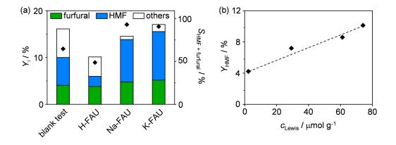
**Figure 1** a) Product yields observed in the CFP of glucose over protonic and sodium- and potassium-exchanged faujasite-type zeolites. Results of the blank test are included for comparative purposes. b) Correlation between the yield of HMF and the concentration of Lewisacid sites.
