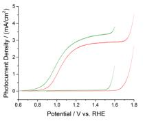
Figure 1 Performance of an unmodified hematite-titania photoanode (shown in red) and after the addition of the amorphous Fe<sub>20</sub>Cr<sub>20</sub>Ni<sub>20</sub>O<sub>x</sub> overlayer (shown in green). Conditions: 1M NaOH (pH=13.6), 10 mVs<sup>-1</sup> scan rate, uncorrected for ohmic losses. The dark currents are shown in the corresponding colors. Photocurrents correspond to AM 1.5 G 100 mWcm<sup>-2</sup> simulated solar light.
