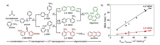
**Figure 1.** a) Reaction network for the synthesis of MDA. b) Linear correlation between the MDA yield and the product of external surface area and Brønsted acidity observed over conventional and hierarchical USY zeolites of varying composition and mesoporosity.
