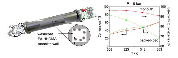
**Figure 1**Illustration of the three-phase semi-hydrogenation of functionalized acetylenes over the monolithic catalyst. The plot highlights the superior selective performance of the monolith compared to a packed-bed reactor in the conversion of 1-hexyne.
