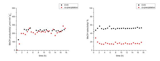
Fig. 1: Methanol productivity and selectivity over CuO-ZnO/Al2O3synthesized via CVD ( $\blacksquare$ ) and co-precipitation ( $\bigcirc$ )
