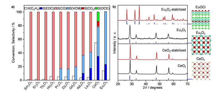
**Figure 1** a) Performance of lanthanide oxides in ethylene oxychlorination at 723 K. b) X-ray diffractograms of as-prepared and stabilized  $CeO_2$  and  $Eu_2O_3$  catalysts.
