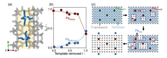
**Figure 1** (a) Location of TPA<sup>+</sup> within the straight pore channels of a ZSM-5 zeolite, (b) the distribution of Ps components as a function of the template removal, (c) a possible mechanism for the SDA removal based on the insights gained by PAS.
