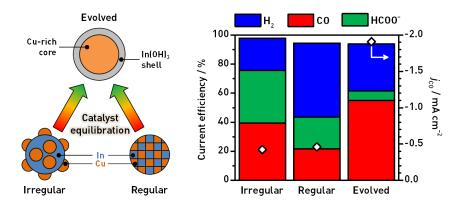
**Figure 1** Cu-In nanoalloy catalysts converge after an equilibration phase towards a common core-shell-like structure with high activity and selectivity for the reduction of CO (performance shown at -0.6 V vs. RHE in CO<sub>2</sub>-saturated 0.1 M KHCO<sub>3</sub>).
