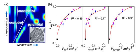
**Figure 1** (a) An example contour plot derived by DHS of argon sorption and (b) the correlation between the mesopore geometry and the effectiveness, based on the out-diffusion of *ortho*-positronium ( $F_{vac}$ ).
