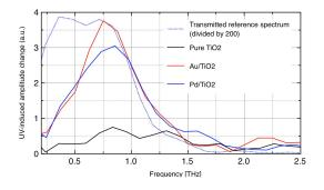
Figure 1: UV-induced transient terahertz absorption in three different titania samples. Compared to pure titania, the presence of noble metal nanoparticles leads to a 4 to 5-fold increase in the number of conduction band electrons.
