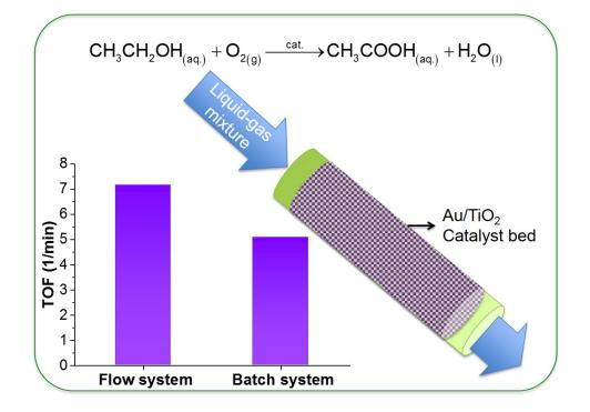
**Figure 1.** Illustration of the 3-phase reactor. The use of a continuous system improves turn over frequency while enhancing the safety of the operation.
