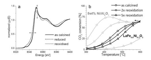
**Figure 1:** a) In situ Ni K-edge XANES on  $LaFe_{0.8}Ni_{0.2}O_3$  during redox cycle; b)  $CO_2$  hydrogenation after a number of simulated catalyst regeneration (reoxidation) cycles for conventional Ni/Al<sub>2</sub>O<sub>3</sub> and  $LaFe_{0.8}Ni_{0.2}O_3$  catalysts
