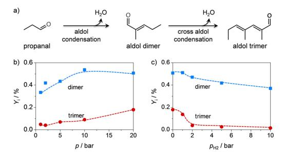
**Figure 1** a) Reaction pathways for the vapor-phase conversion of propanal over base catalysts at 673 K. b) Impact of total pressure and c) partial pressure of hydrogen on the product yield over alkali metal-grafted zeolites.
