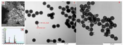
Figure 3: SEM (A), EDS (B) and TEM (3C) showing core-shell Sn@SiO<sub>2</sub>, 3(D) showing Sn@SiO<sub>2</sub>@C after thermal treatment
