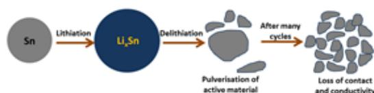
Figure 1: Pulverization of the active material
